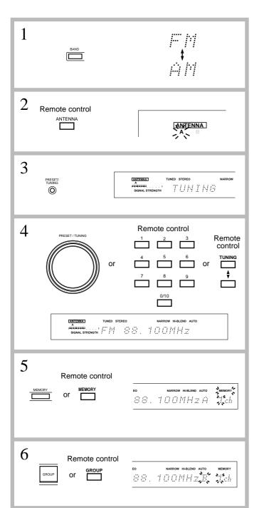
In order to listen to a radio broadcast, first tune in the radio station, then set it. The radio station can be selected in two ways: by using the auto-tuning function or by directly entering the station's frequency. When tuning in the radio station, refer to page 12 for more information on how to get the best reception possible.
